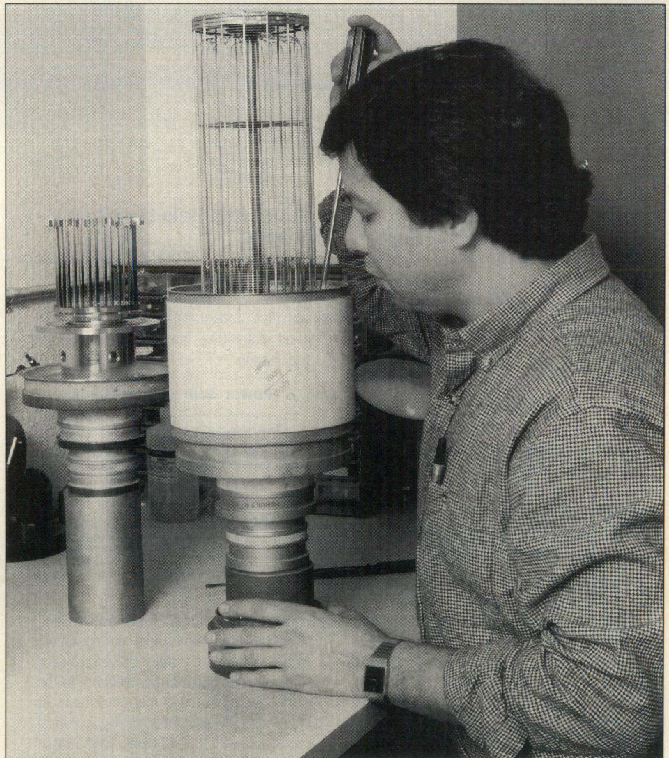
An example of a rebuilt power grid using the platinum clad wire.
